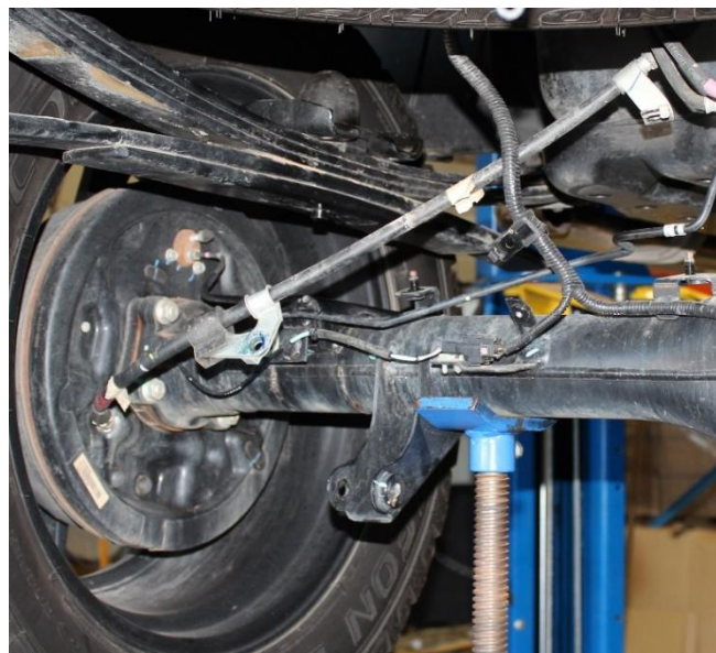
Picture 3: Raising Block Installation
