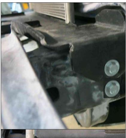
16. Fix left side of the bracket to insert nuts M10 with bolts M10x50 and washers No. 10. DO NOT TIGHTEN YET.
