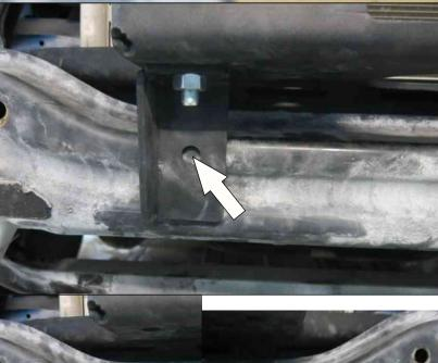
17. Mount brackets #2 and #3 to winch bracket using bolts M12x30, nuts M12 and washers #11. Mark future apertures on the front cross-bar.
