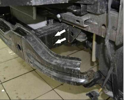
13. Increase the size of the 2 apertures on left side of underframe by drilling them to 10mm diameter.
