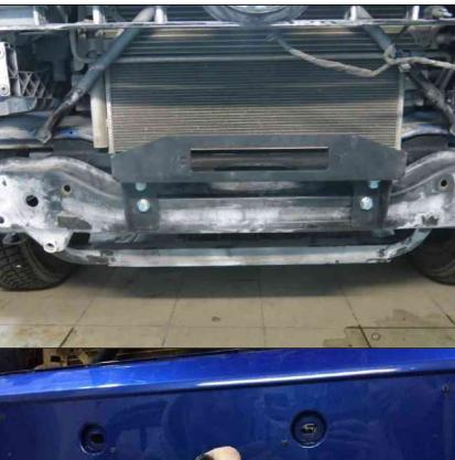
19. Mount brackets #2 and #3 to the winch bracket using bolts M12x30, nuts M12 and washers #11.
