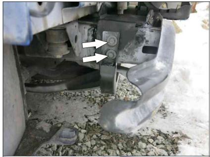
14. Install the winch bracket to underframe. On right side, place winch bracket under the original skid plate bracket. Slightly screw OE bolts of skid plate. DO NOT TIGHTEN YET.
