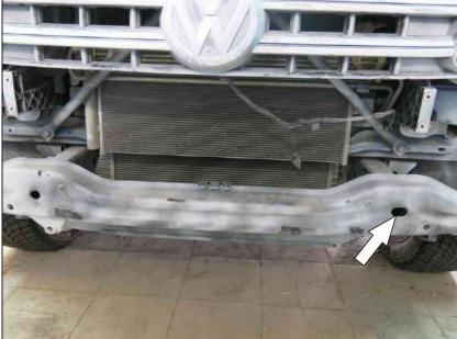
15. Insert nuts M10 into OE aperture in underframe.
