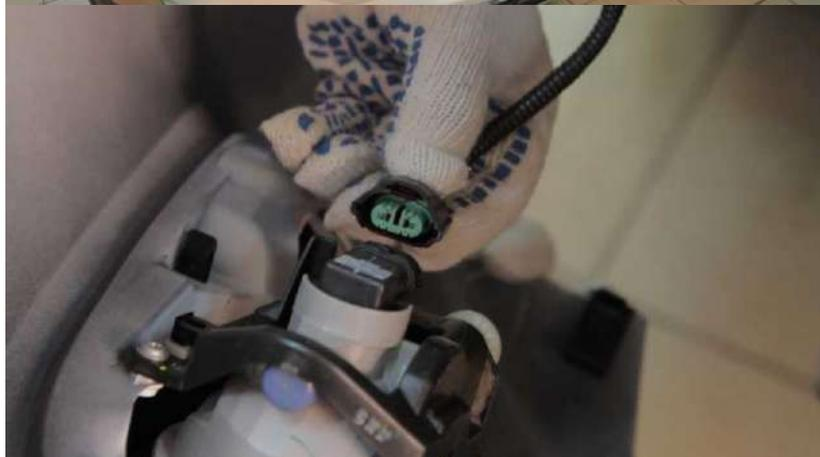
7. Remove the washer hose and disconnect wires.
