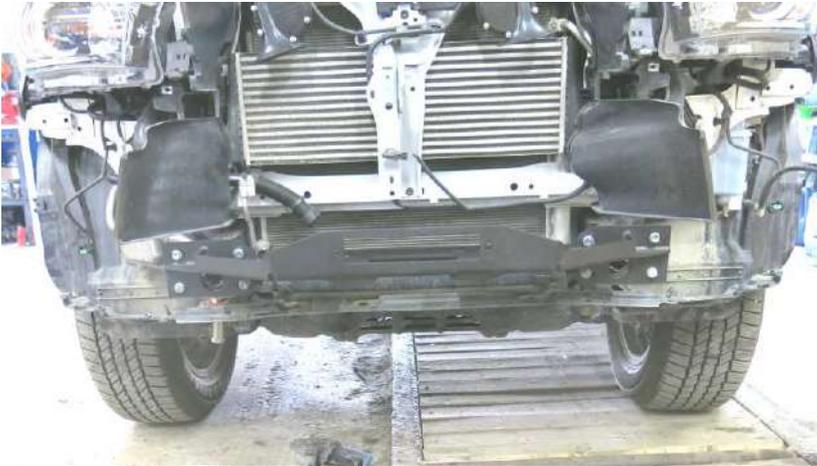
12. Fix winch bracket to insert nut M12 (4). Place insert nut into hole in the chassis and fix it using bolt M12x30 (7), washers (15 and 16).
