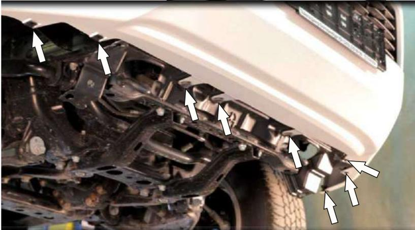
4. Remove lower screws as shown.
