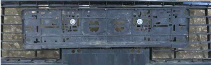
17. Mount license plate frame to the bumper using brackets (3), screws M6x50 (8) and washers (13)
