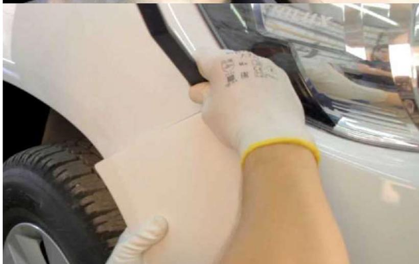
6. Remove the bumper by pulling the bumper towards you holding the sides
