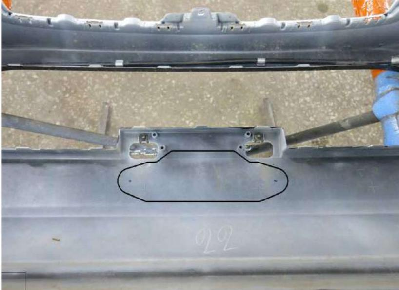
14. Temporarily place plastic bumper back to its place to mark cutting line for the fairlead
