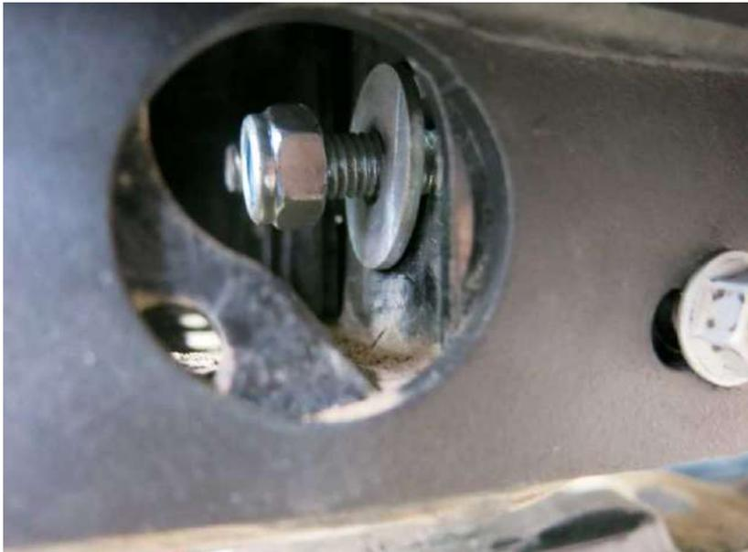
13. Fix winch bracket using bolts M12x30 (7), nuts M12 (11), washers (15 and 17).
