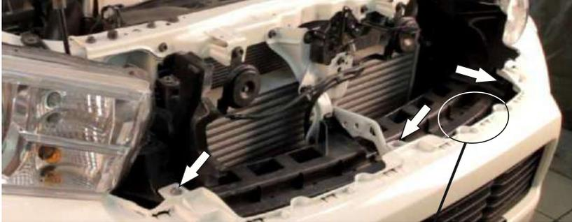
3. Remove shown screws and plastic clips.
