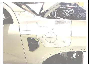
8. Cut out the supplied guard template and fit the template to the fender making sure it is aligned correctly.
