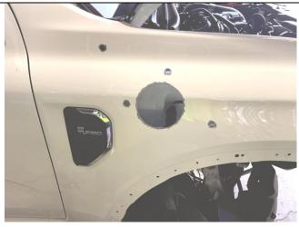
9. Remove all sharp edges from the holes then remove the template. Treat all raw/exposed edges with a rust preventative product or similar.
