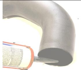
25. Apply a liberal amount of neutral cure silicone to the inside surface of the airbox connector at the snorkel end.
