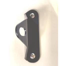
16. Remove the "A" pillar bracket from the snorkel body and secure to the "A" pillar using <sup>3</sup>/<sub>4</sub>" x 8G stainless steel PK screws supplied.
