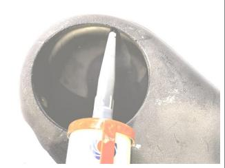
24. Apply a liberal amount of neutral cure silicone to the inside surface of the snorkel end of the intermediate tube.
