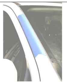
10. **Positioning of the "A" pillar bracket on the vehicle:-** Using a protective tape, mask the RHS "A" pillar as indicated to prevent potential damage
