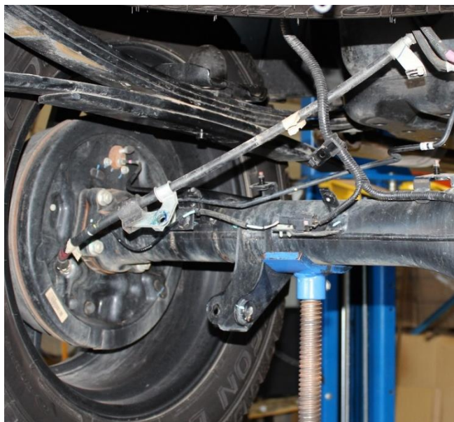
Picture 2: Raising Block Installation
