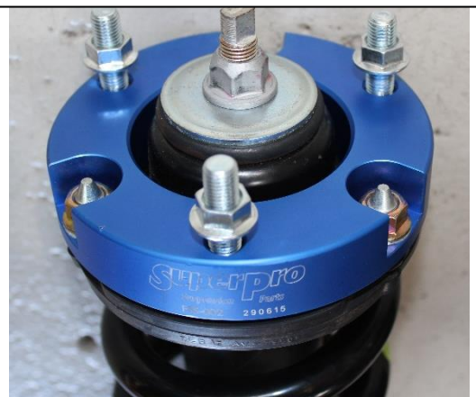
Picture 1: Picture of strut spacer on strut
