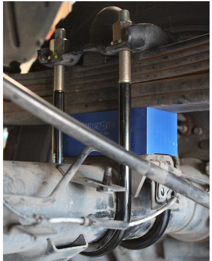
Picture 4: U-bolt tightened
