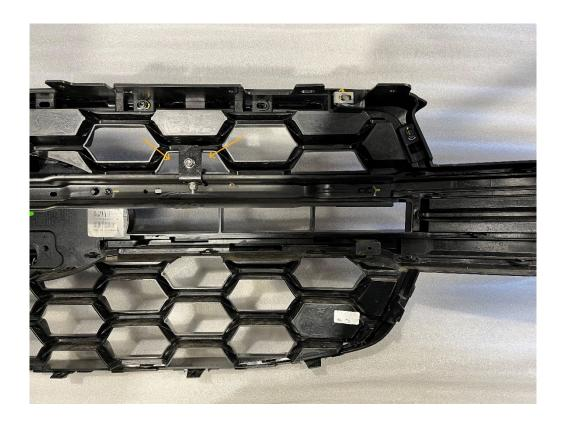
• Once brackets fixed in position, fix stay bars to brackets. Re fit grille at the bottom half only so that top of grille can be pulled forward for routing wiring.
