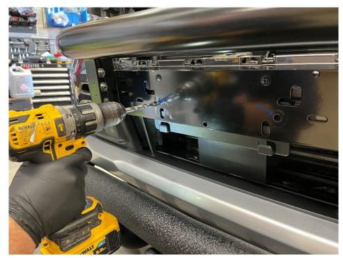
• Drill & fix stay bar bracket in the centre of the vent opening shown below, repeat for the opposite side. *Note – metal support bar can be removed for ease of drilling.*
