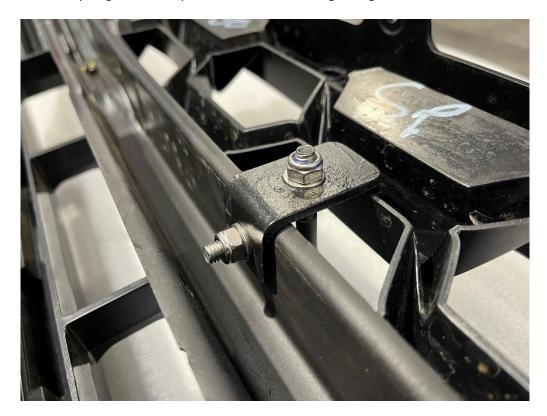
• Before installing lights, two lights require holes to be tapped M6 in the hole location shown below. These tapped holes are for the stay bars.
