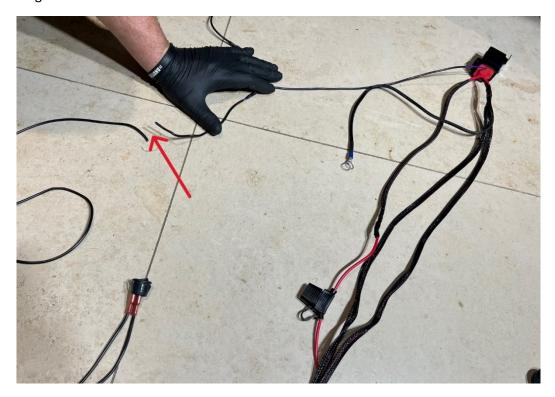
• Signal wire needs to be routed into the cab of the vehicle and connected to 'Pos Light' wire connection. Red wire shown below shows a location for routing through bulkhead, this is near side.
