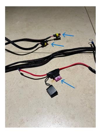
Remove the switch from both looms by cutting both switch wires. (Leave a safe length on
