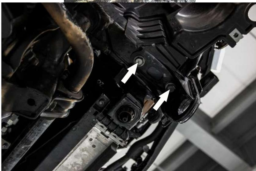
20. Unscrew 2 tension bolts of standard
