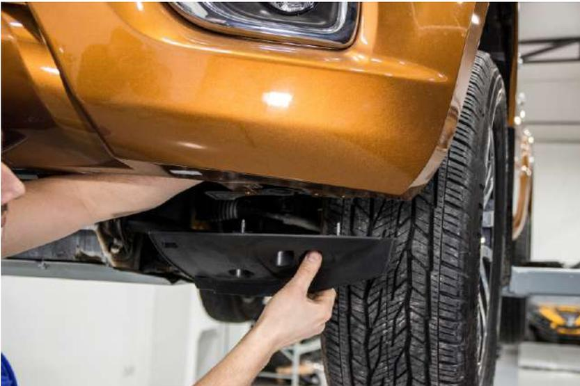
11. On the bumper inside unscrew 2 retaining nuts of the bumper skirt side and dismantle the bumper skirt side.
