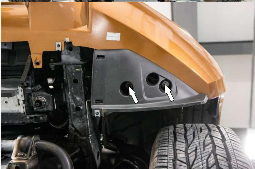
10. Unscrew 2 tension bolts of the bumper skirt side on the vehicle's left and right.
