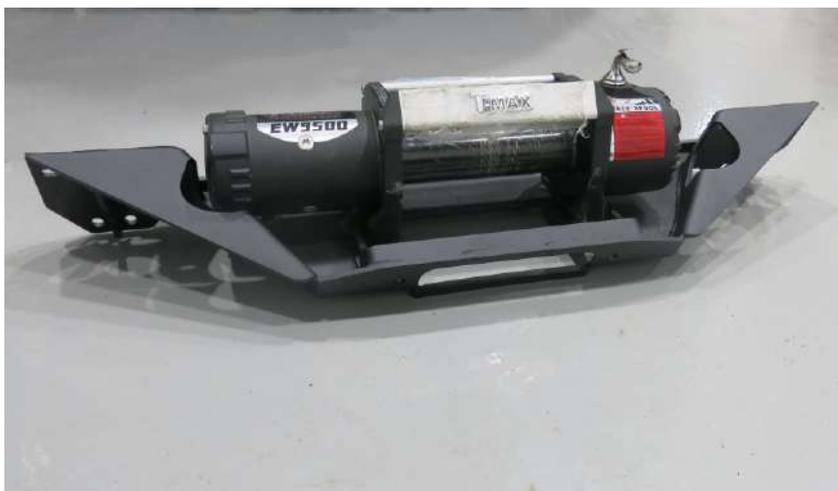
29. Remove the winch bracket from the vehicle, install the winch and pad eye onto the bracket and secure with bolts from the set of winch and pad eye.
