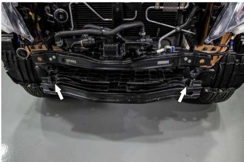
18. Remove the air intake clips.
