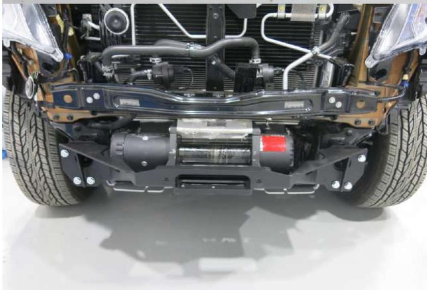
30. Install the winch bracket onto the vehicle. See paragraph 25.
