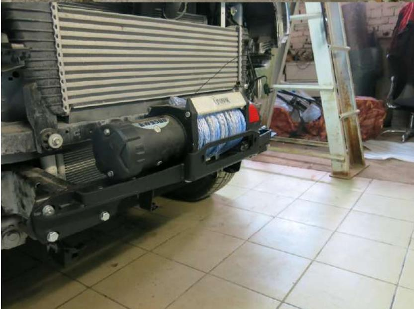
20. Mount the winch and fairlead to the bracket using the bolts supplied with the fairlead.
