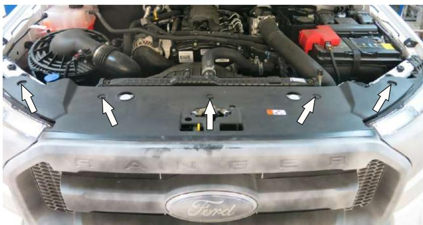
5. Remove 4 screws out of radiator grill.
