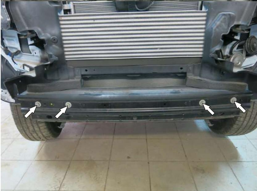
13. Remove 4 bolts out of front bar.
