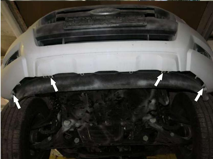
4. Remove 4 screws out of lower lip of the bumper.
