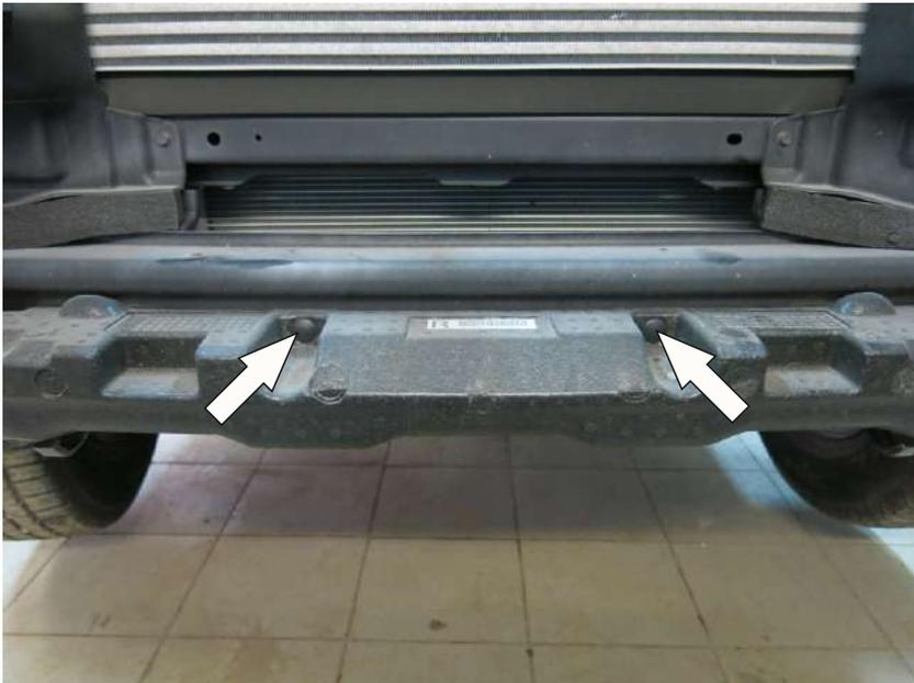
11. Remove the plugs out of the panel.
