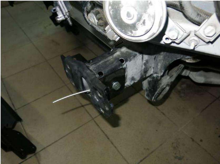
17. From outside of the chassis, mount outer bracket (2) from both left and right side. Fix them with bolts M10x30 (6), washers (8) to insert nuts (5).
