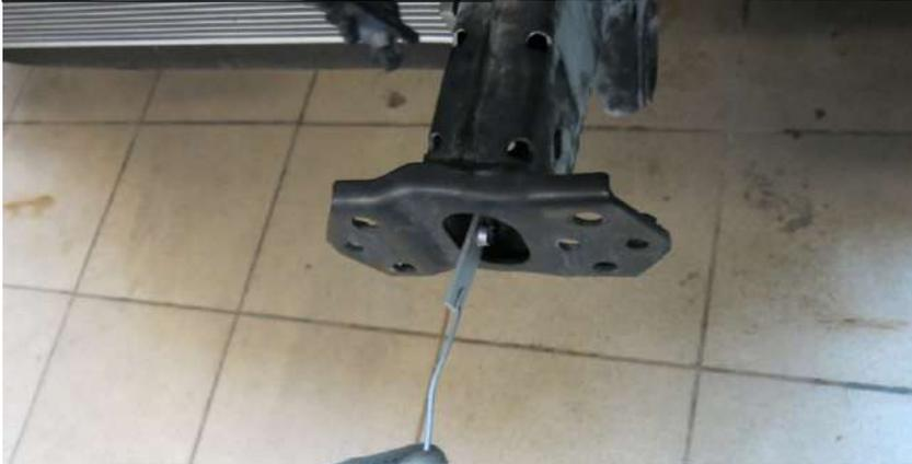
15. Insert nuts (5) into the underframe.
