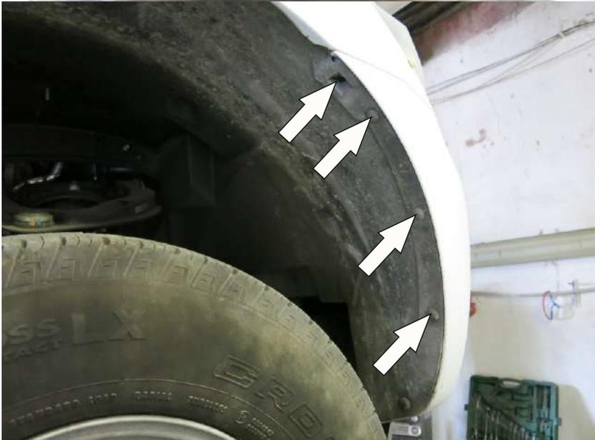
3. Remove 4 screws from inside of the fenders on each side of the vehicle.
