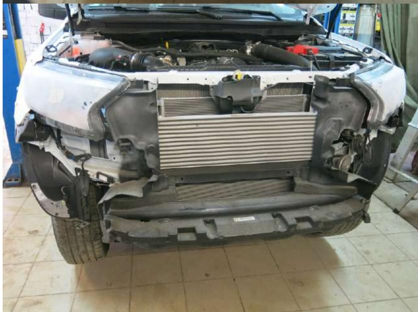
10. Deinstall the bumper. Pull the bumper towards you holding the sides.
