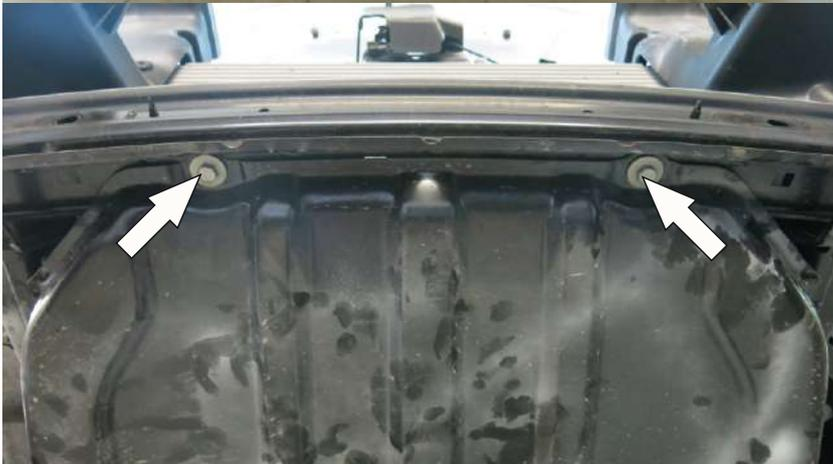
12. Remove 2 bolts out of skid plate.
