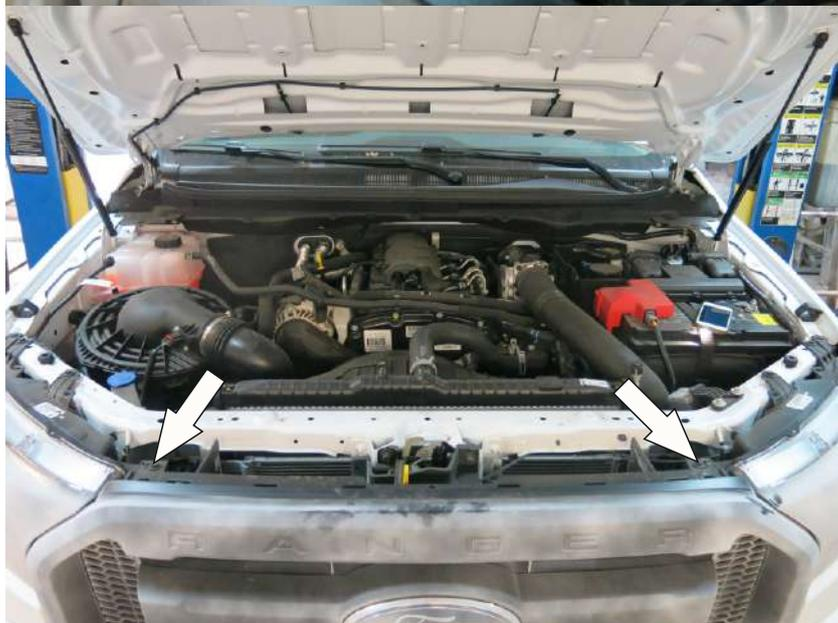
7. Remove 2 screws out of radiator grill.
