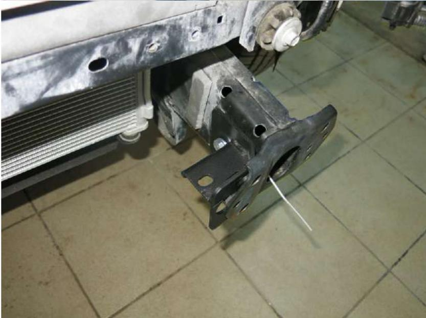
16. Mount inner left bracket (3) to the left side chassis. Fix it with bolts M10x30 (6), washers 8 to insert nuts (5).
