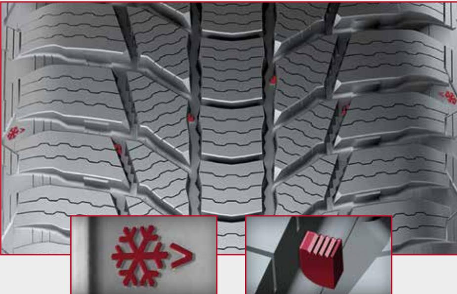
The Winter TWI (Tread Wear Indicator) indicates a remaining tread depth of 4 mm.
