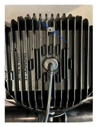
• Instal the lights onto the mounting bracket using the fittings provided with the lights. \*Note\* – the penny washer arrowed red below is provided in the WR46-FITTINGKIT
