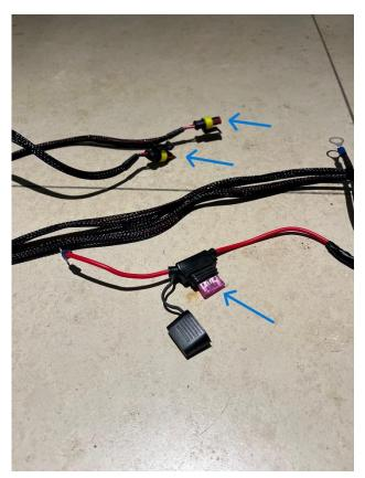
• Signal wire needs to be routed into the cab of the vehicle. Red wire shown below shows a location for routing through bulkhead, this is near side.
