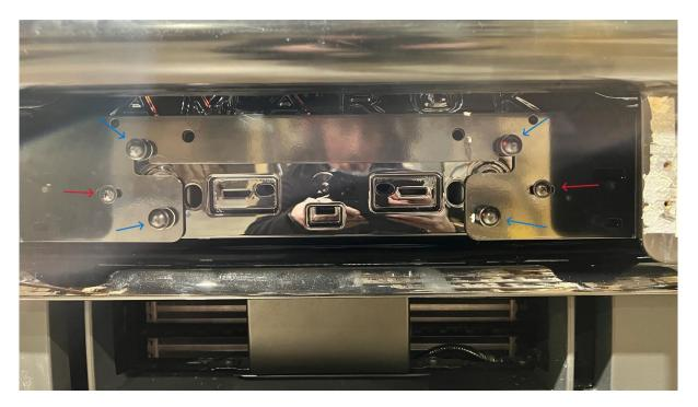
• Remove fixings so that top half of the grille can be pulled forward, remove support bar. Drill & fit the stay support L bracket to the support bar as shown below, the measurement from the outer edge to the end of support bar is 237mm - *illustrated with blue arrow below*. Repeat for other side. Now fix stay bars to these brackets.
