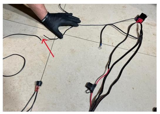
• Remove the switch from both looms by cutting both switch wires. (Leave a safe length on one) Both switch wires on the loom need to be connected together so that they become one signal wire.
