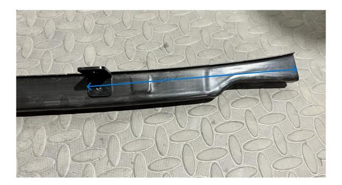
• Before installing lights, two lights require holes to be tapped M6 in the hole location shown below. These tapped holes are for the stay bars.
