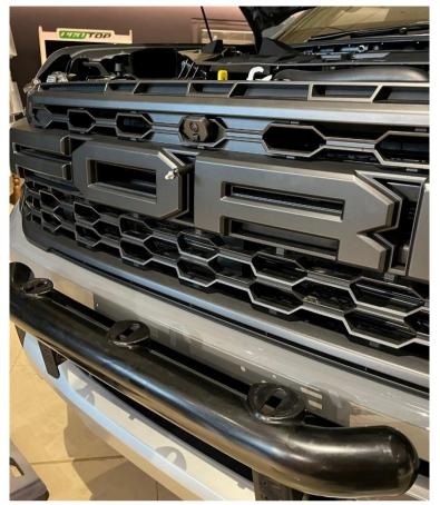
• Before installing lights, tap the rear of one of the lights M6, (hole location shown below). This light is for the centre, and the tapped hole is for the stay bar.
