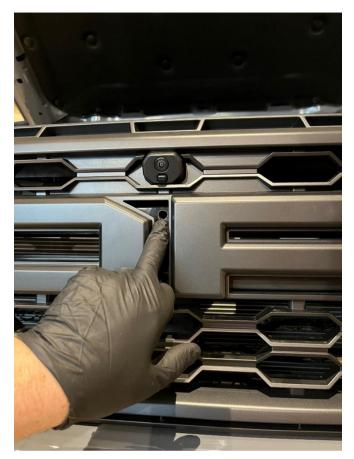
• Remove the plastic trim from the top of the grille and pull the top of the grille forward slightly. You will now be able to fit the stay be and have access to secure in place from behind the grille.
