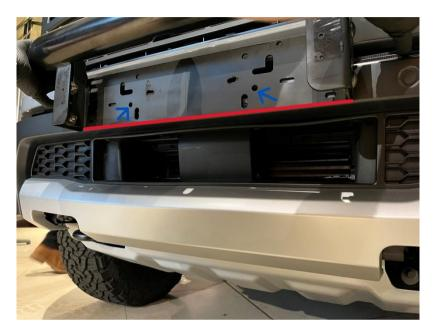
• Drill 8mm holes through bumper and right through including the metal plate that is at the rear of bumper, but being cautious as to not drill into radiator.
