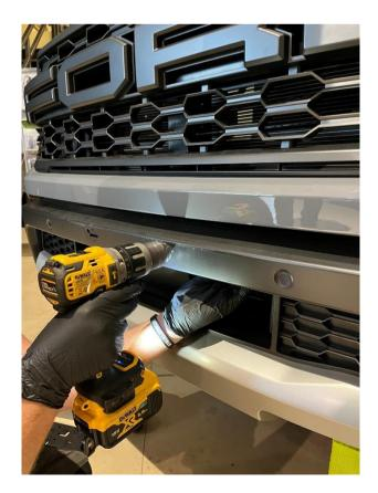
• A hole needs to be drilled for fitment of the centre stay bar, drill an 8mm hole in the centre of the grille, and just below the front camera as shown;
