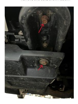
• Fit bracket using the same bolts as shown below.
