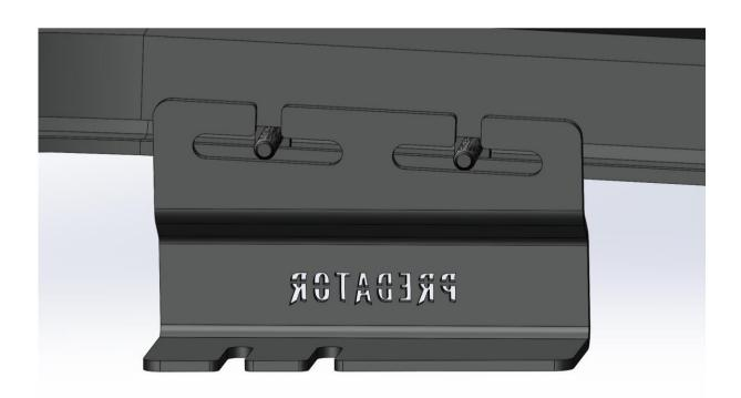
Once lowered, slide T-Slot bolts to either side of bracket and fit nuts (Don't fully tighten at this stage) Repeat for each mounting bracket.
