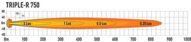
Generated from BSI (British Standard Institute) lamp photometric test data: On Road measurement data
