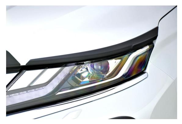
If the ambient temperature of the working area is below 10°C it is recommend that application of heat is used to promote adhesion. A heat gun (shown in "Tools Required" section) is sufficient to provide enough heat to allow the adhesive tape to set.
