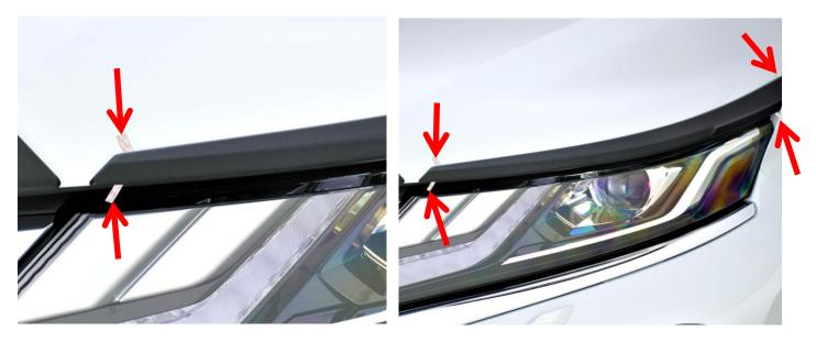
Once happy with the positioning of the head lamp trim pull each of the tabs to fully expose the adhesive tape on the rear of the trim. Press firmly around the edge of the head lamp trim to ensure the adhesive has made contact with the bonnet.
