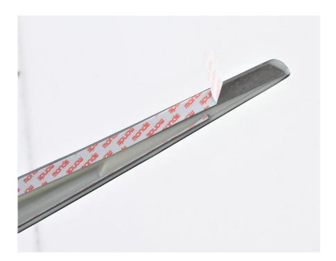
Offer the head lamp trim into position on the bonnet of the vehicle leaving the tabs exposed.
