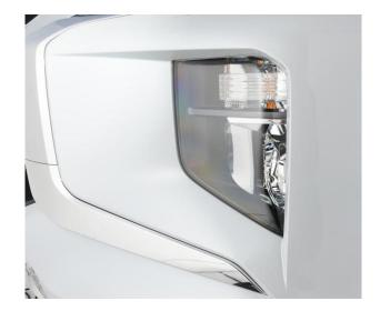
Take the first fog lamp trim out of the box and peel back a small tab on each section of the adhesive tape on the rear of the trim as shown in the image below.
