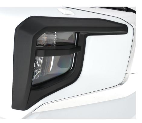
If the ambient temperature of the working area is below 10°C it is recommend that application of heat is used to promote adhesion. A heat gun (shown in "Tools Required" section) is sufficient to provide enough heat to allow the adhesive tape to set.
