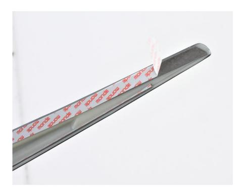
Offer the fog lamp trim into position on the front bumper of the vehicle leaving the tabs exposed.
