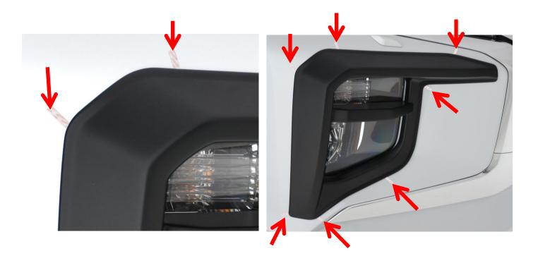
Once happy with the positioning of the fog lamp trim pull each of the tabs to fully expose the adhesive tape on the rear of the trim. Press firmly around the edge of the fog lamp trim to ensure the adhesive has made contact with the front bumper.
