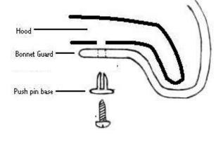
3. Fit the plastic "W" clips to the 4 holes at the outer edge of the Bonnet Guard. Apply the supplied rectangular pieces of anti-abrasive tape on edge of bonnet where plastic fastening "W" clips secure the Bonnet Guard.
