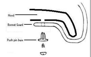
3. Fit the plastic "W" clips to the holes at the outer edge of the Bonnet Guard. Apply the supplied rectangular pieces of anti-abrasive tape on edge of bonnet where plastic fastening "W" clips secure the Bonnet Guard.
