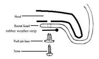
5. Apply the anti-abrasive tape on edge of hood where plastic fastening clip secures the Bonnet Guard near the fenders. Use the supplied alcohol prep-pads to cleanse the area first.
