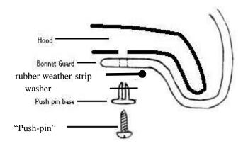
5. Apply the anti-abrasive tape on edge of hood where plastic fastening clip secures the Bonnet Guard near the fenders. Use the supplied alcohol prep-pads to cleanse the area first.
