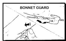
6. Snap the supplied plastic "W" clip into hole position on Bonnet Guard as shown, over the anti-abrasive tape.
